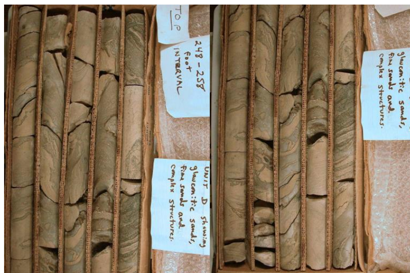
Figure 20. Core photos showing jumbled and deformed Cambrian strata from the southern edge of the Rock Elm central uplift - from WGNHS archives.
