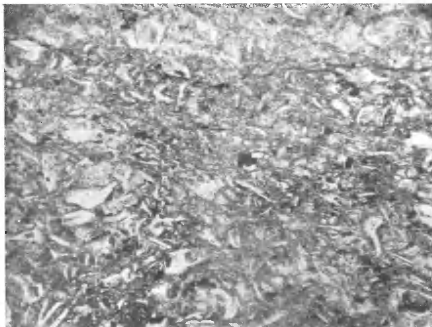
Figure 10. Shard structures in rhyolite from Ninth Street and Winton Avenue, Wausau. Magnification approximately 140x.
