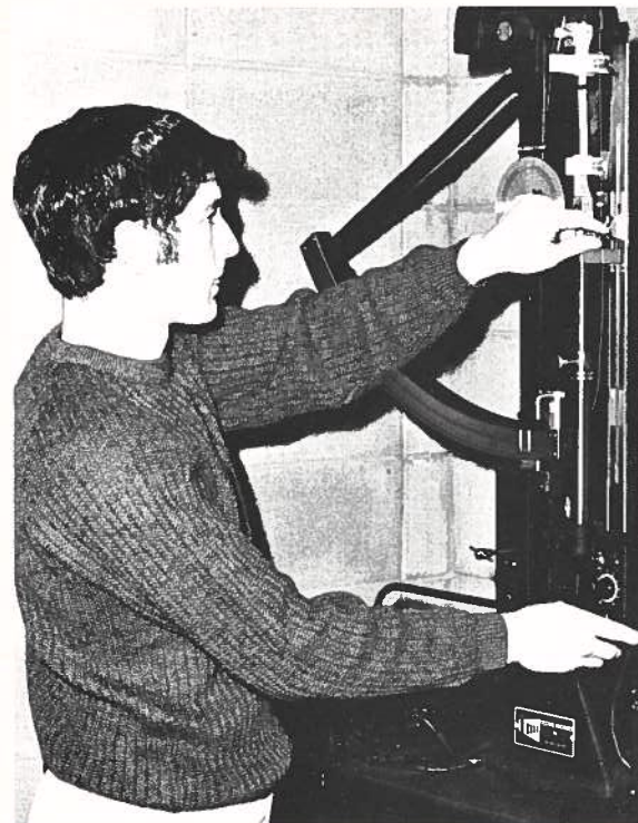
Student evaluating the tensile strength of a paper sample in the environmentally controlled Physical Testing Lab.
