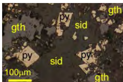
Figure 1. Pyrite (py) and siderite (sid) in oxidized GIF (gth = goethite). Reflected light.
