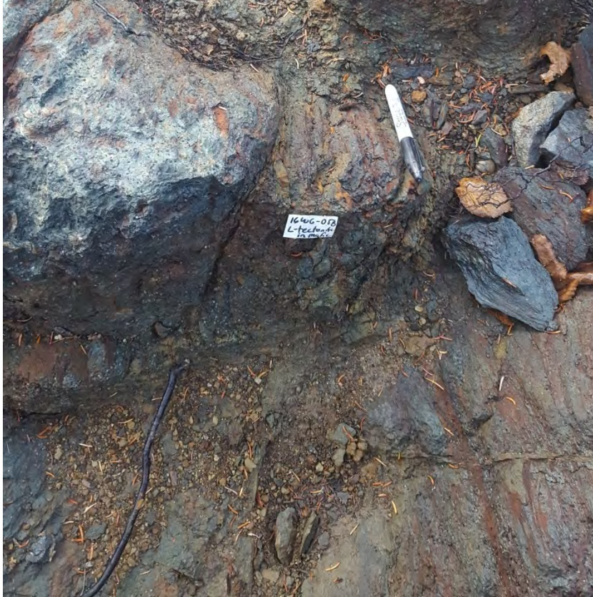
Figure 7 - Characteristic stretching lineation of the Wawa Gold Corridor preferentially partitioned in a mafic dike (William Gold Zone)
