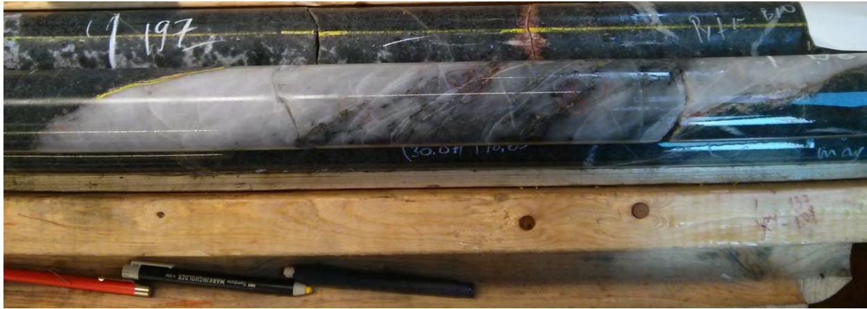
Figure 13 - Quartz tension vein with visible gold in the footwall of the Surluga Deposit Drilling intersection contains 53.2 g/t gold over 1 m
