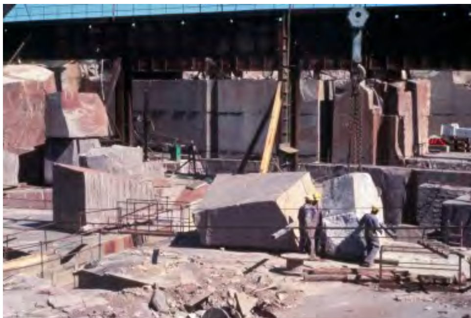
Figure 11. Granite dimension stone blocks being removed from Cold Spring Quarry in 1982.
