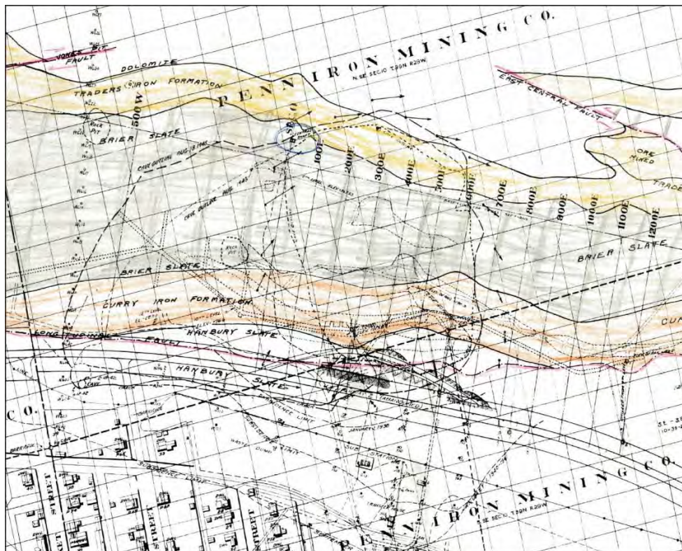
Figure 13. Plat of the Central Vulcan are in 1938. Geological interpretation and mine sites including subsidence area.
