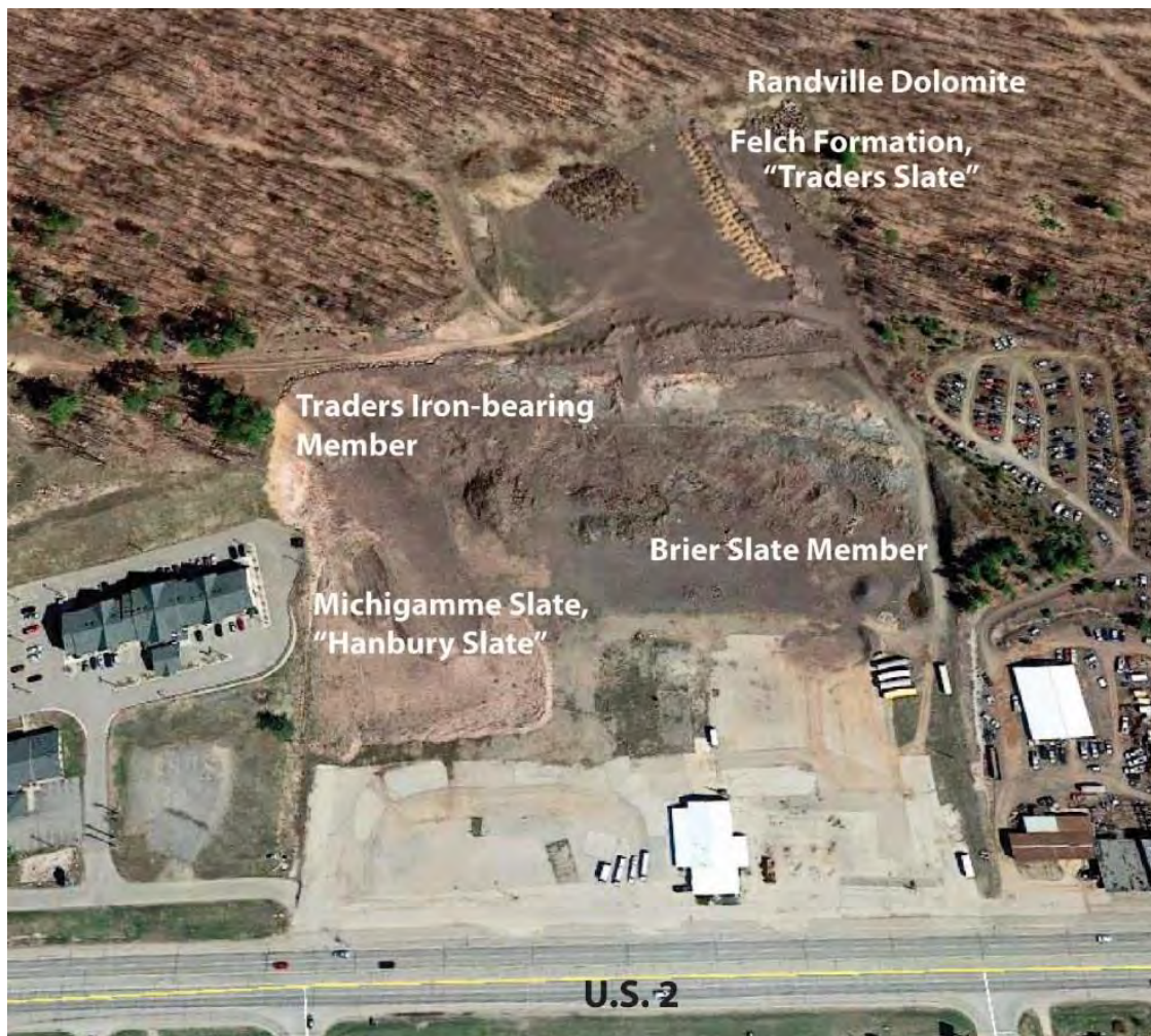
Figure 25. The Keel Ridge mine area. Geologic units are as indicated in USGS Professional Paper 513, Plate 1 (Bayley et al., 1966). Excavation reveals the northwest-striking formations that include the upper part of the Felch Formation (“Traders Slate”), Traders Iron-bearing Member, Brier Slate, and Michigamme Slate (“Hanbury Slate”). The formations face to the south and dip to the north at 80°- 90°.
