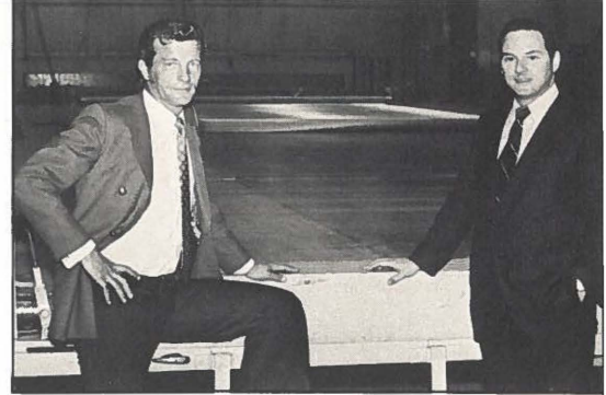
West Coast Wire's Plant Superintendent Peter Slaney, left, with Motorways Sales Rep Dennis Caporale. Behind them is the stretching frame where finished wires are stretched to the exact size required by the paper manufacturer.
